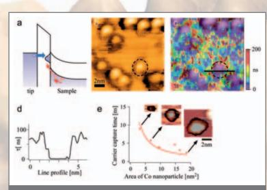
Fig. 3 (a) Schematic of the carrier recombination mechanism via the gap states. (b) STM image of Co nanoparticles/GaAs. (c) Overlap of color-scale two-dimensional mapping of decay constant obtained over the surface in (a). (d) Cross section of the decay constant along the line in (b). (e) Hole capture time as a function of nanoparticle size.
